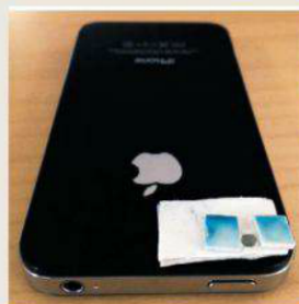
DOUBLE-SIDED TAPE and a glass lens turn a smartphone into a field microscope. The two images above show parasitic worm eggs under a traditional microscope (left) and with the iPhone version (right).
